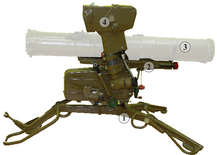
1 - Tripod 2 - Portable launching units 3 - Containers with missile 4 - Optical sight
